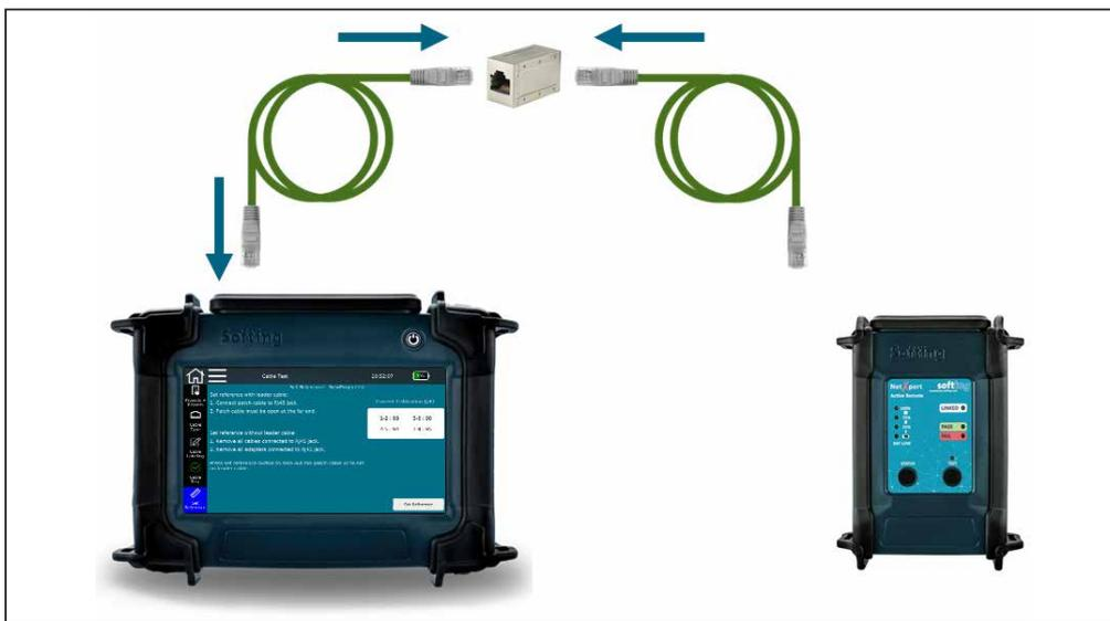
Figure 25 – Test setup for setting the reference
