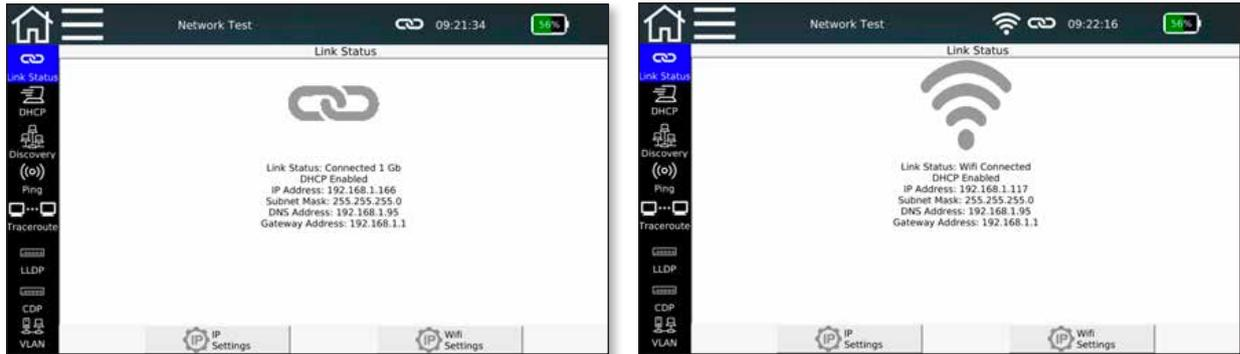
Figure 27 – Link Status, wired connection (left) or via WiFi (right)
