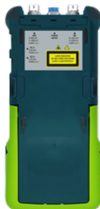
Modul FQ GLASFASER QUAD MULTIMODE 850/1300 nm SINGLEMODE 1310/1550 nm
