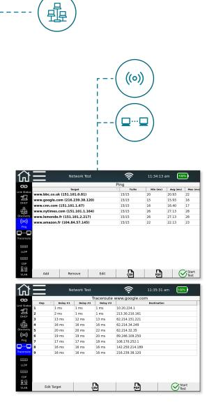
The ping function allows you to check the accessibility of network devices such as servers and printers as well as Internet connectivity.
