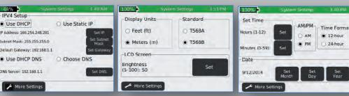
Display Units, Brightness and **IPv4** Parameter Setup Wiremap color scheme Setup
