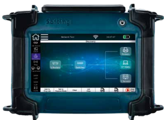
For network discovery, simply connect NetXpert XG to a switch via copper, fiber, or WiFi with the local unit
