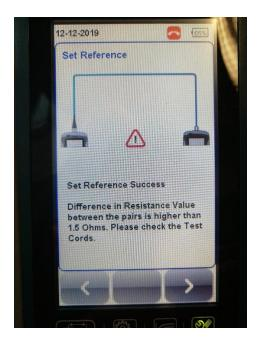
This can cause bad test results, particularly in Resistance and Return Loss values!
