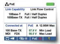
The CableMaster 800/850 will also identify the "Connected at" status and display the physical connection condition:
