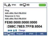
Press the Test button to select an IP address then press the Test button again to ping the selected IP
