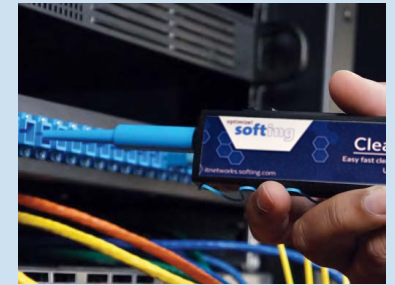
Remove cap for cleaning adapters and bulkheads
