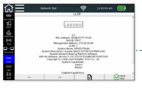
Display of switch port data via evaluation of the Link Layer Discovery Protocol (LLDP) or Cisco Discovery Protocol (CDP)
