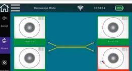
With the fiber optic microscope, the connector end faces can be quickly and easily checked and subjected to an automatic "Pass/Fail" evaluation in accordance with IEC 61300-3-35. This is automatically combined with the qualification results in a detailed test report.
